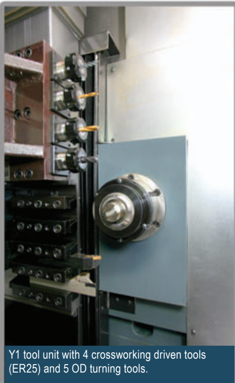
42mm back spindle with C-axis
