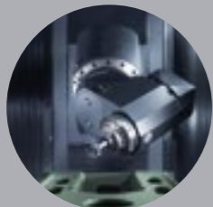
THC_ B axis head Maintain the same tool center point across the full range -15°/+195°
