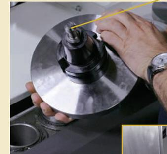
*Kitamura's integrated work ID system employs an IC chip on the bottom of each pallet allowing for storage and communication of pallet work data quickly and accurately to the easy-to-operate pallet scheduling sub menu.*
