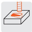
Fresatura in rampa
