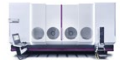
Y-Z travels Y 1100 mm - Z 1000 mm (Option 1200 mm) Tool holder (ZV EXTREME) SK 50 • BT 50 • HSK A-100
