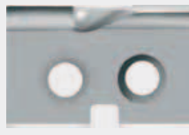
Blind hole insert* (HSS-E/PM or HSS-E) without center point
