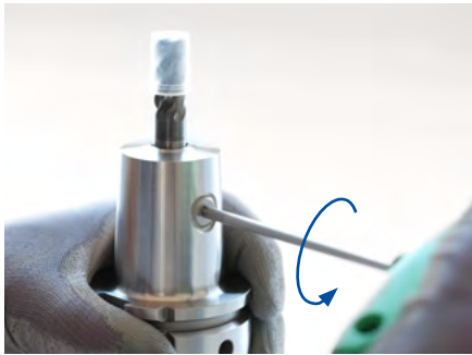
1. Loosen the clamping screw by turning it counter clockwise.
