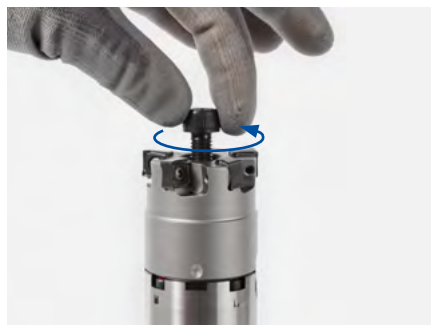
1. Unscrew the milling cutter clamping screw from the threaded bore and remove it.
