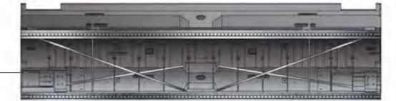
Crossbeam Cross Section: 1030 mm x 1305 mm
